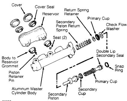
Fig. 16: Chrysler Motors Composite Master Cylinder Courtesy of Chrysler Motors
