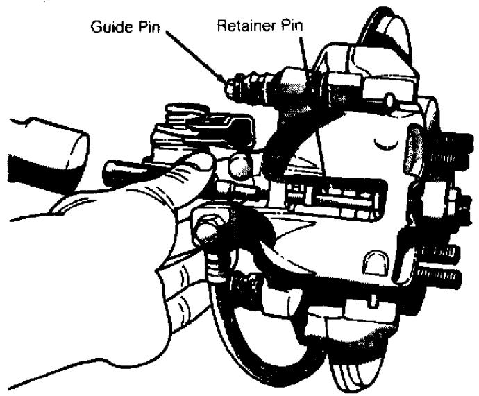
Fig. 10: "C" Body Rear Brake Assembly Courtesy of Chrysler Motors.
