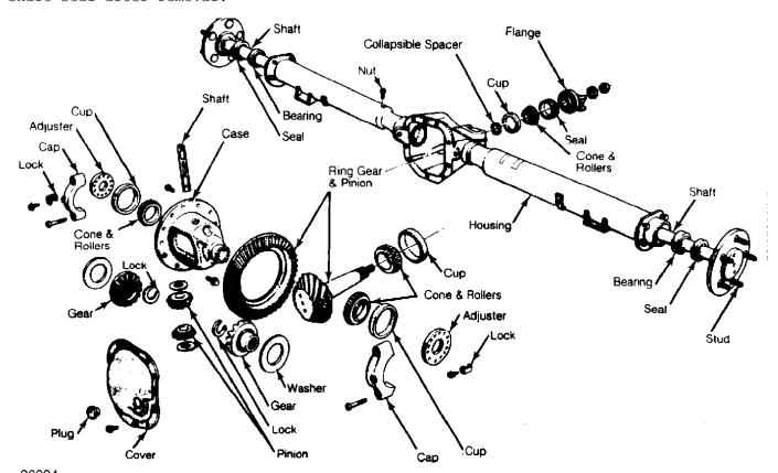
Fig. 11: Chrysler Corp. 7 1/4" Rear Axle Assembly Courtesy of Chrysler Motors
