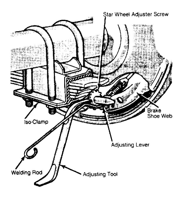
Fig. 3: Adjusting Rear Brake Shoe-to-Drum Clearance
