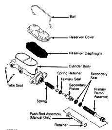
Fig. 15: Typical Cast Iron Tandem Master Cylinder Courtesy of Chrysler Motors
