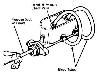
Fig. 5: Bench Bleeding Master Cylinder Courtesy of Chrysler Motors
