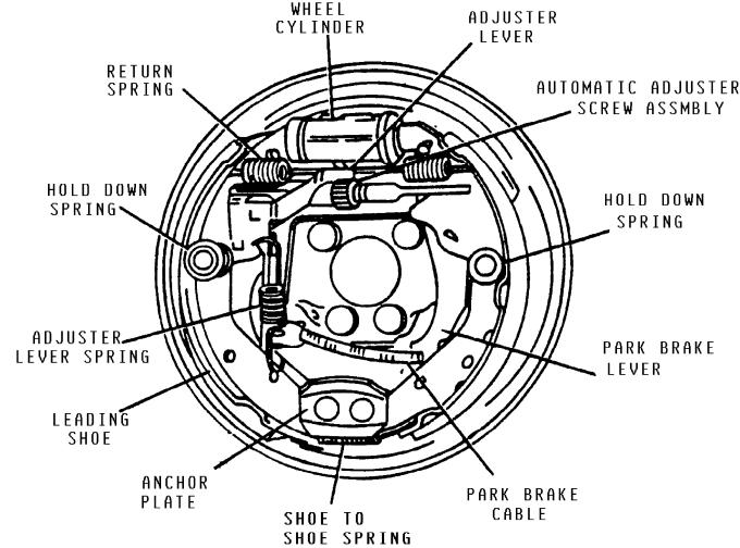
Fig. 1: Kelsey Hayes Automatic Adjuster Brake Assembly Courtesy of Chrysler Motors
