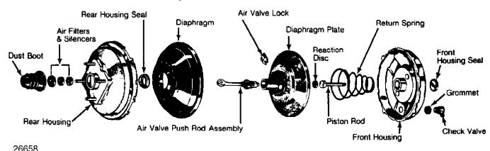
Fig. 6: Exploded View of Bendix Single Diaphragm Booster Courtesy of Chrysler Motors
