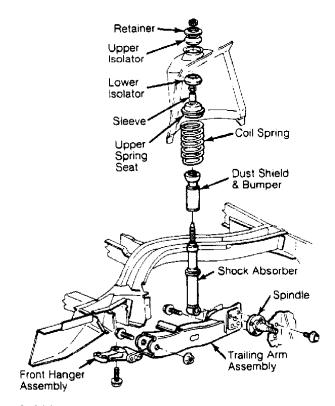
27014 Fig. 13: Rear Suspension Assembly (Charger, Omni, Horizon & Turismo) Courtesy of Chrysler Motors
