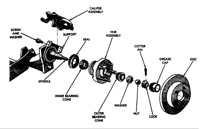
Fig. 9: Exploded View of Daytona Rear Brake Assembly Courtesy of Chrysler Motors.
